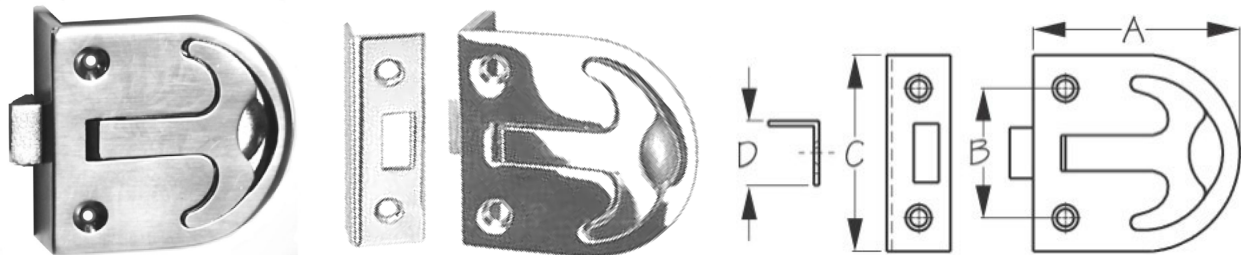
#43.831S Flush Slam latch, Pull type. Anchor style lift ring; strike plate included. Pull Out to release. Dimensions: 2 7/16" (A) x 1 1/2" (B) x 2 1/4" (C) x 3/4" (D) Door thickness: 3/4". 316 Stainless Steel Satin Finish
