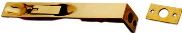
#55.668 series flush bolt 3/4" x 6"; depth: 1 5/16"; throw: 5/8"; Solid brass with stainless steel pins and springs. Positive locking in open or closed position Marine grade.
