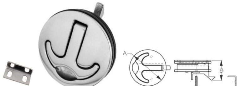
#43.9714 Slam latch 2 7/16 diameter (A); drill hole 2 3/16 inch, distance (B): 1 3/8" material up to 5/8" thick; 316 polished stainless steel
